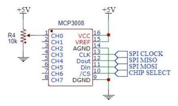
Fig. 12. MCP 3008 ADC Schematic [21]
