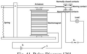
Fig. 41. Relay Diagram [39]
