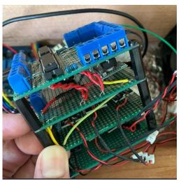
Fig. 36. 3 Layered PCB Design [1]
