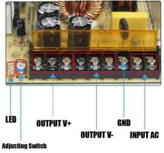
Fig. 43. Power supply's Terminals [40]
