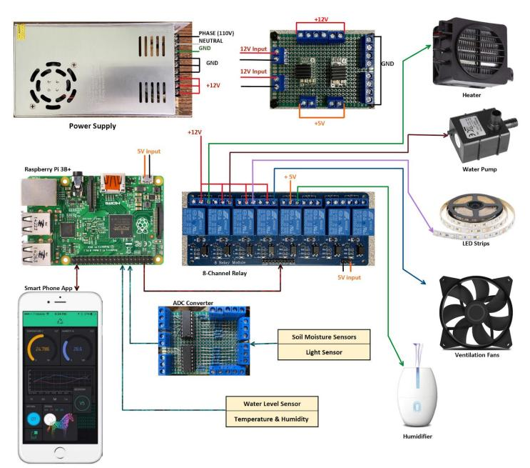
Fig. B2. Spring 2020 Prototype Hardware Connections [1]
