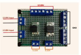
Fig. 44. Power Distribution Board [1]
