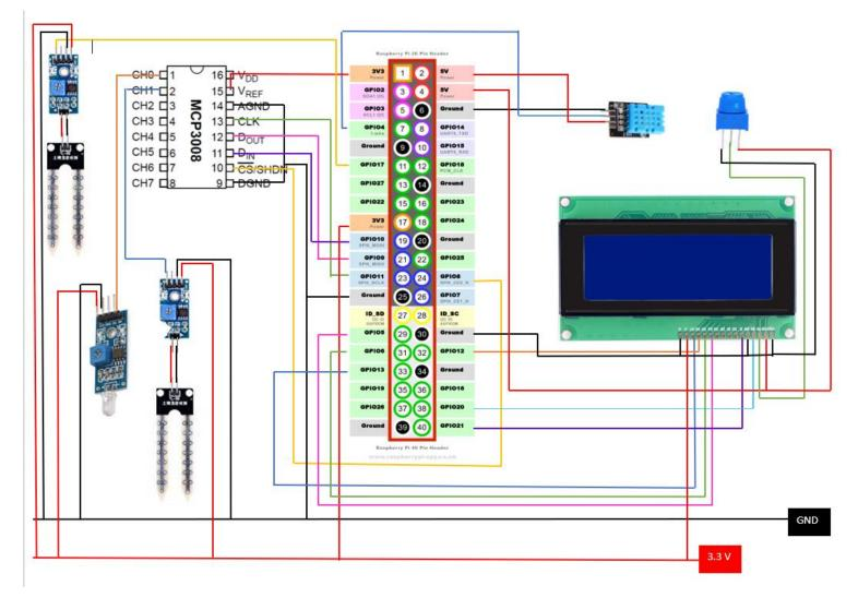
Fig. B1. Fall 2019 Raspberry Pi Connections Schematic [1]
