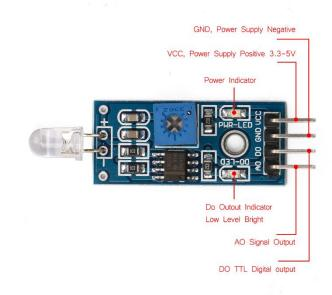
Fig. 10. DROK 200033 Light Level Sensor [19]
