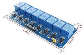
Fig. 40. SunFounder 8-channel Relay [38]
