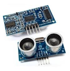
Fig. 33 Ultrasonic sensor [32]
