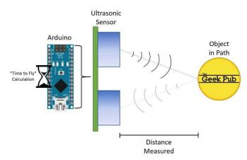
Fig. 34. Ultrasonic Sensor Working Principle [33]
